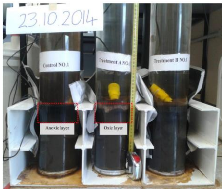
Fig. 7. The color change at sediment-water interfaces in the column experiment after 127 days. Treatment A and treatment B are ONMZ and ONMS, respectively. The photo was taken off for the picture.
